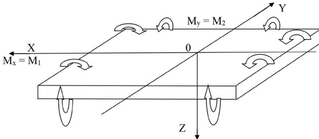
Figure 2: Bending moments on the fixed positions of basaltic filter.
