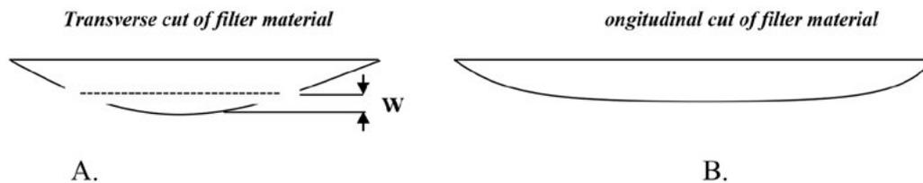
**Figure 1:** The conventional form of the filter in longitudinal and transverse sections.
