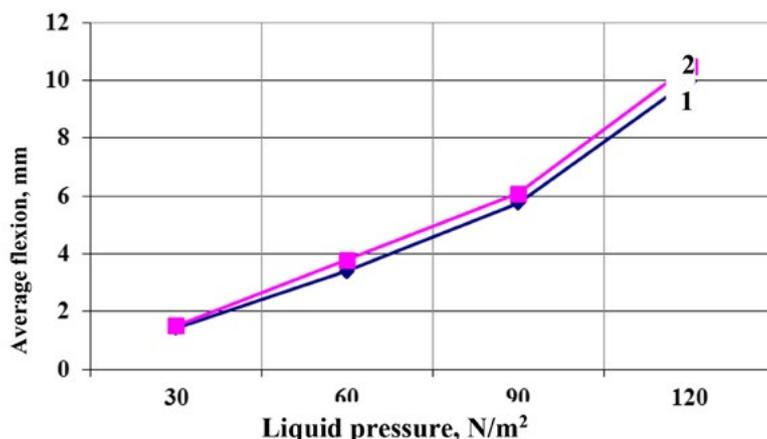
**Figure 3:** Graphs of the dependence of basalt filter bending on the fluid pressure force: 1. Theoretical indicators. 2. Experimental indicators.
