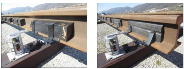
(a) (b) **Figure 1**. Rail dampers: (a) TATA Steel; (b) Vossloh [6].
