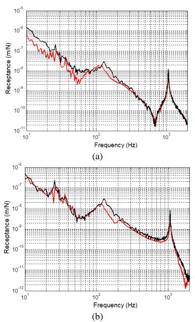
**Figure 5.** Rail receptance: (a) at middle; (b) above sleeper; black line – without dampers, red line – with dampers
