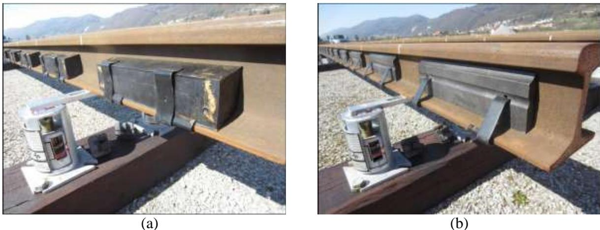
**Figure 1.** Rail dampers: (a) TATA Steel; (b) Vossloh [6].
