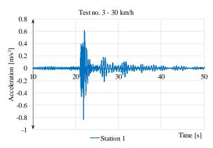
**Figure 10.** The accelerogram for the component 2 of the  $3^{rd}$  test (30 km/h)
