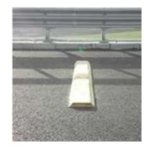
**Figure 7.** Ridge made from a wood board and 45° bevels
