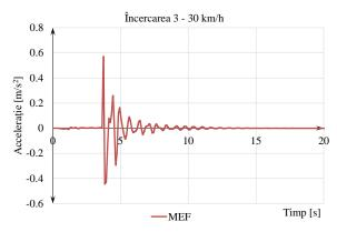
**Figure 22.** Acceleration time-history obtained from FEM analysis equivalent to test no. 3 - 10ad case no. 2 (30 km/h)
