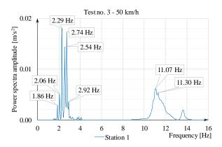
**Figure 16.** The power spectra of the accelerogram for the component 3 of the 3<sup>rd</sup> test (50 km/h)
