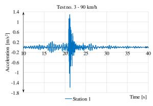
**Figure 13.** The accelerogram for the component 5 of the 3<sup>rd</sup> test (90 km/h)
