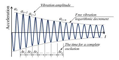
Figure 8. The theoretical free vibration response of a SDOF system
