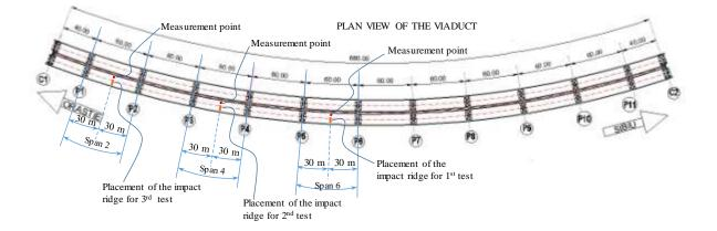
Figure 1. The general plan view of the viaduct, the measurement points position and the placement of the impact ridge
