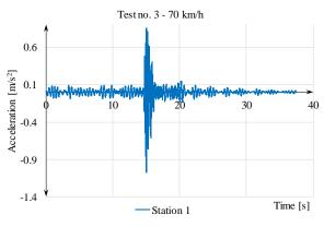
**Figure 12.** The accelerogram for the component 4 of the  $3^{rd}$  test (70 km/h)
