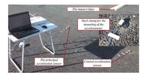
**Figure 3.** The placement of the acceleration sensors in the 3<sup>rd</sup> span of the viaduct
