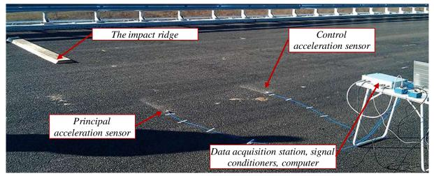
Figure 2. The equipment for the accelerations measurement
