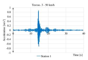
**Figure 11.** The accelerogram for the component 3 of the  $3^{rd}$  test (50 km/h)
