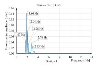
Figure 14. The power spectra of the accelerogram for the component 1 of the  $3^{rd}$  test (10 km/h)
