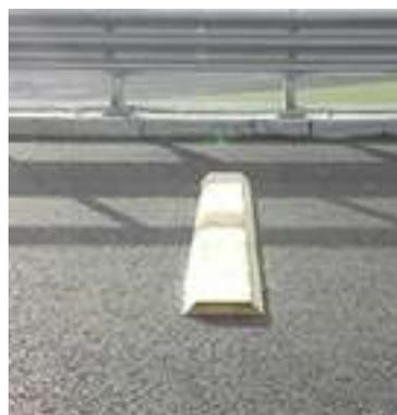
**Figure 7.** Ridge made from a wood board and 45° bevels
