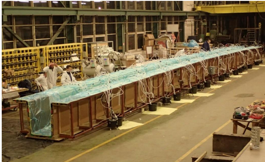
Figure 3. VARTM process of the girder
