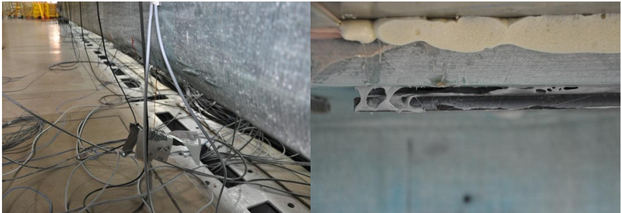
Figure 12. Plastic deformation at the transition zone between the bottom flange and the web in the middle of the girder (left) and the failure of epoxy adhesive joining upper flange and steel plate of shear stud
