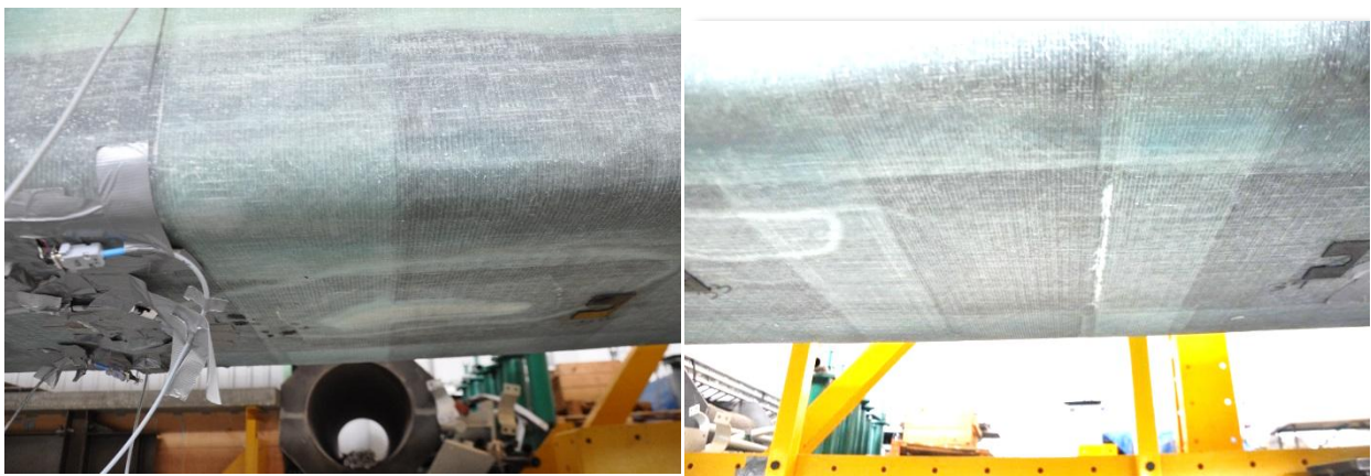
Figure 10. Local delamination of the upper flange in the middle of the girder (the location of structural notch made in the production stage of the girder)
