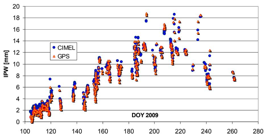
**Fig. 10.** Hornsund IPW from CIMEL-318 measurements and GPS in 2009 (only hours with both measurements available)
