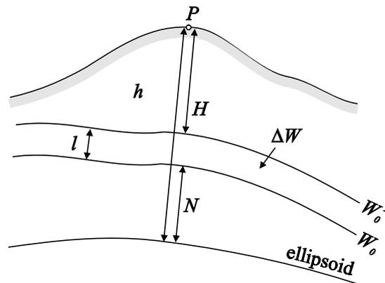
**Fig. 1.** The principle of vertical datum unification
