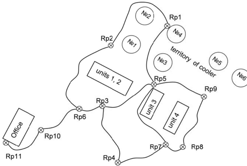
**Fig. 1.** Scheme of height reference network on the territory of Rivne NPP
