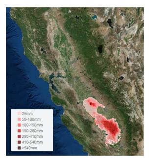
Figure 5. Subsidence contours in the Central Valley of California (image from USGS: https://ca.water.usgs.gov/land\_  ${\tt subsidence/california-subsidence-areas.html)}$
