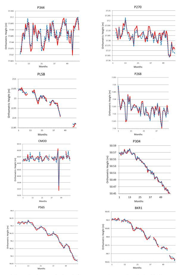
Figure 4. Subsidence at the eight points used in this study after removing seasonal motion. In the graphs, the solid red line represents the original height values and the dashed blue line represents the elevations after seasonal motion is removed. The horizontal axis is scaled in months for five years from 1 to 60, and the vertical axis shows the height in meters.
