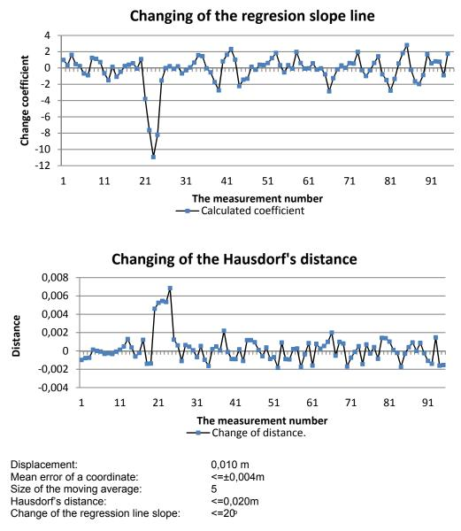
Fig. 6. Results of simulation and analysis
