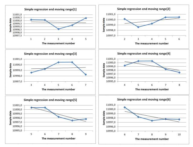
Fig.4. Changing the direction of the regression line based on the following arguments moving average dimension of 5
