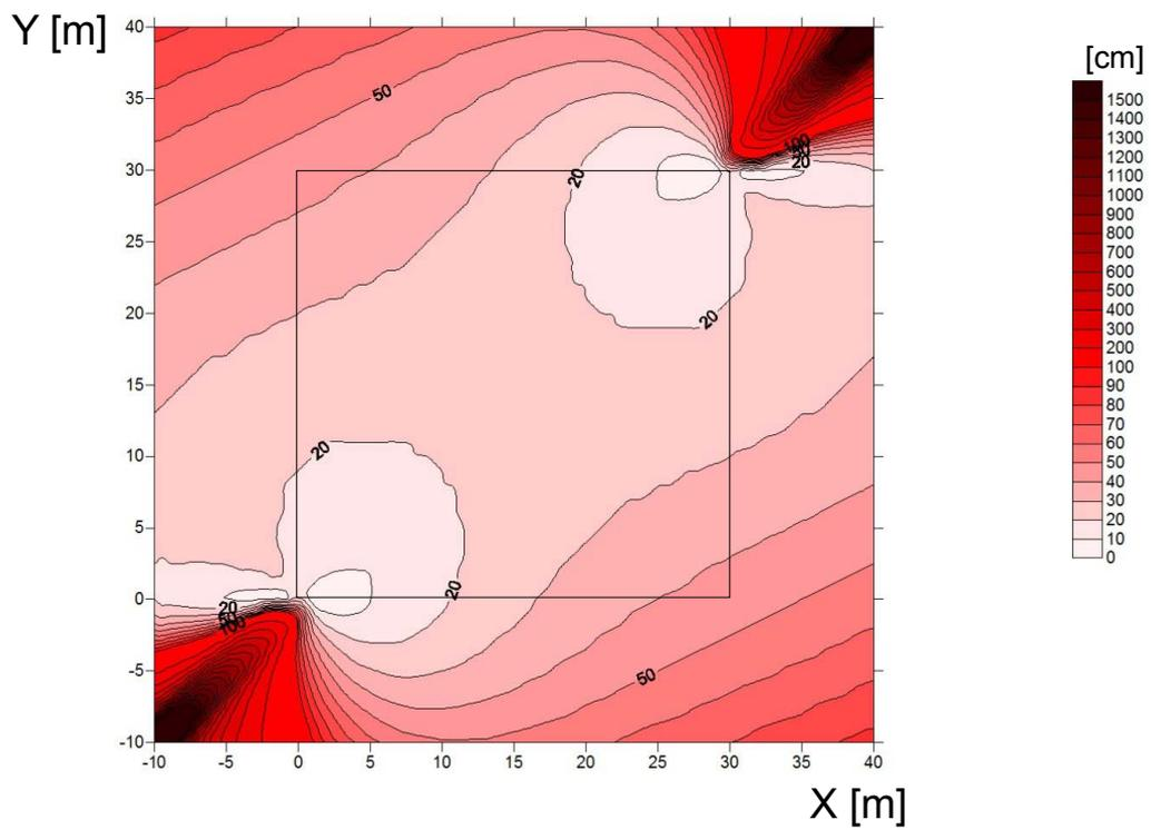
**Fig. 10b.** Distribution of predicted accuracy of the Y coordinate (2 sensor stations mutually turned to each other)
