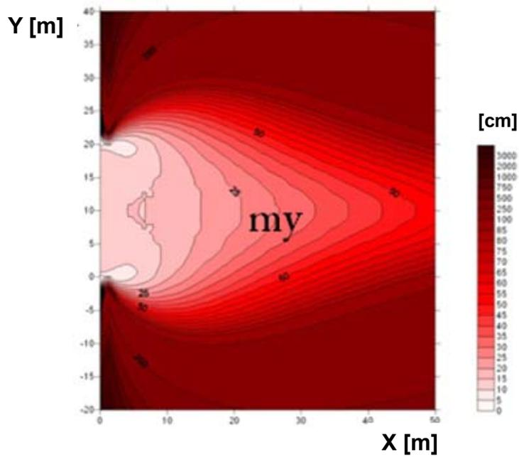
**Fig. 8b.** Distribution of predicted accuracy of the Y coordinate (2 sensor stations turned in the same direction)
