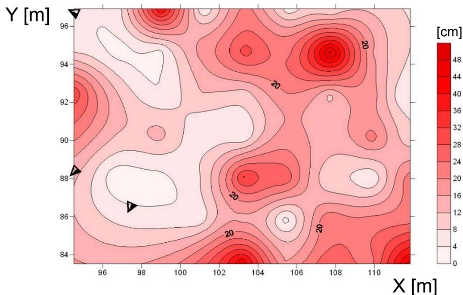
**Fig. 11c.** Graphical presentation of differences  $dz$  between the coordinates obtained from the Ubisense system and the TCPRP 1201+ for a configuration of 3 sensor stations
