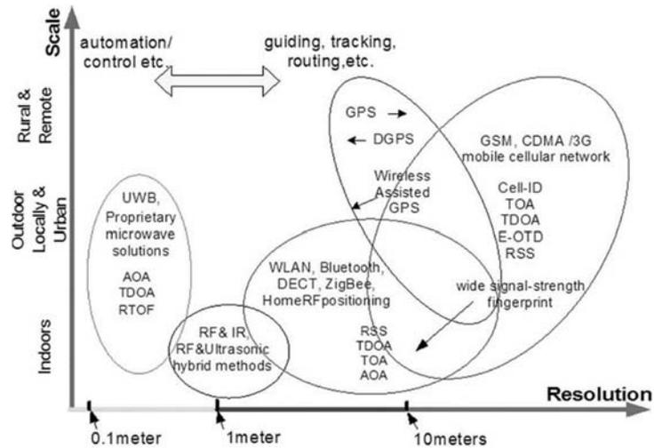
Fig. 1. Positioning systems overview (Liu et al., 2007)
