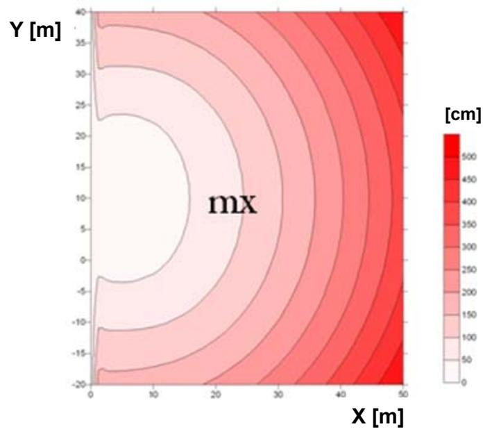
**Fig. 8a.** Distribution of predicted accuracy of the X coordinate (2 sensor stations turned in the same direction)
