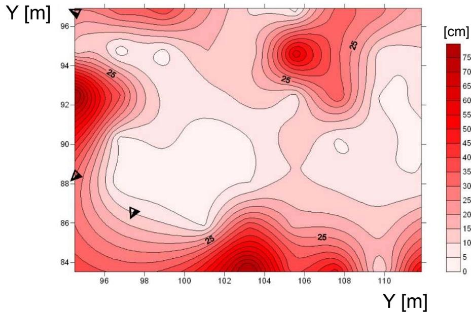
**Fig. 11b.** Graphical presentation of differences  $dy$  between the coordinates obtained from the Ubisense system and the TCPRP 1201+ for a configuration of 3 sensor stations
