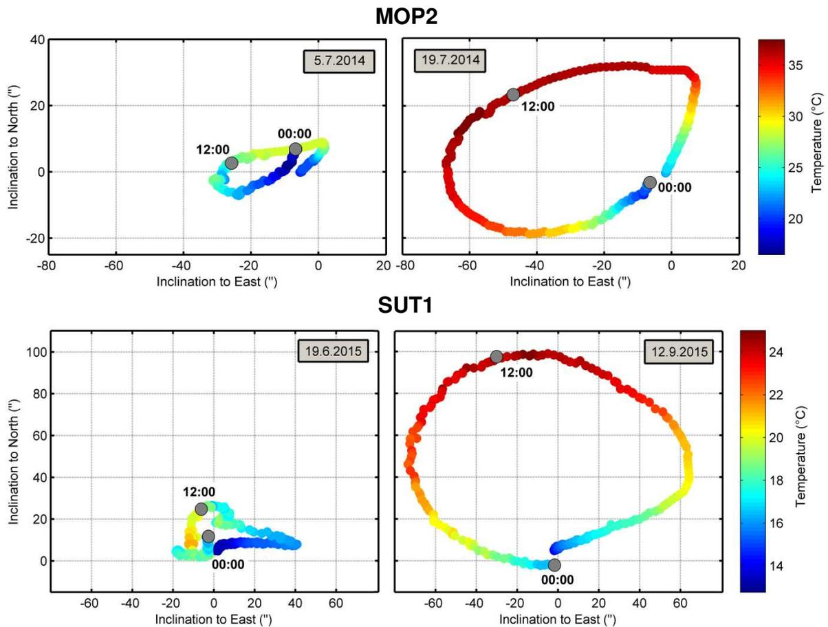
**Fig. 6.** Diurnal cycle of inclination observed at MOP2 and SUT1 in various temperature daily change (temperature course is represented by colours). On the left side are measurements during cloudy days and on the right side the days with all-day sunshine.
