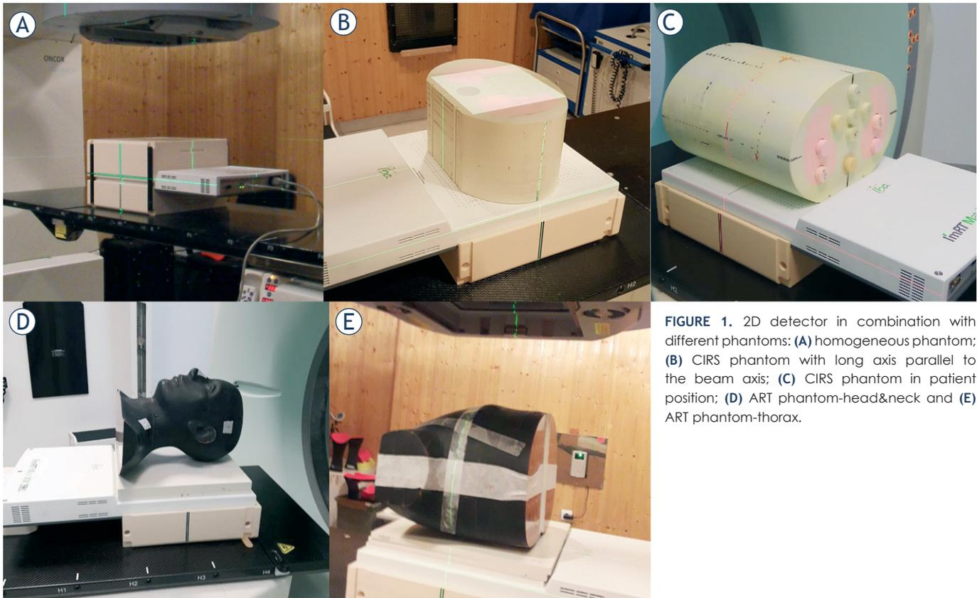
**FIGURE 1.** 2D detector in combination with different phantoms: (A) homogeneous phantom; (B) CIRS phantom with long axis parallel to the beam axis; (C) CIRS phantom in patient position; (D) ART phantom-head&neck and (E) ART phantom-thorax.
