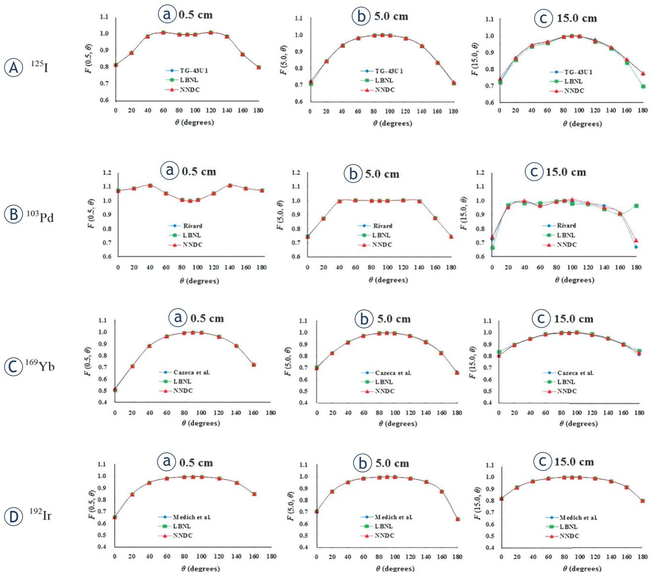
FIGURE 1. 2D anisotropy function values for (A)  $^{125}\text{I}$ , (B)  $^{103}\text{Pd}$ , (C)  $^{169}\text{Yb}$  and (D)  $^{192}\text{Ir}$  sources at  $r = 0.5$  cm (a), 5.0 cm (b), and 15.0 cm (c) distances.
