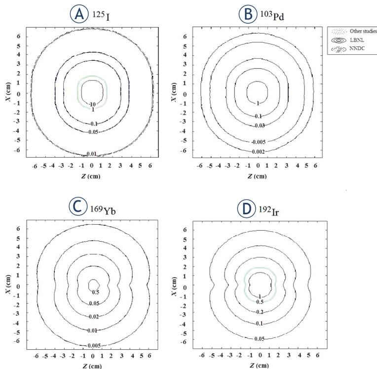
**FIGURE 3.** Isodose curves for (A)  $^{125}\text{I}$ , (B)  $^{103}\text{Pd}$ , (C)  $^{169}\text{Yb}$ , and (D)  $^{192}\text{Ir}$  sources obtained by different photon energy spectra. The contours for various spectra are not clearly distinguishable due to their overlapping.
