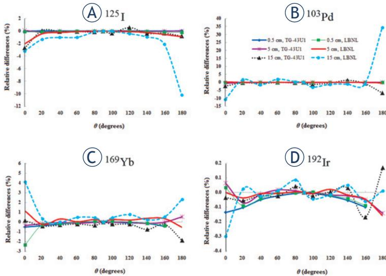
**FIGURE 2.** Percentage differences (%) between the 2D anisotropy function obtained from National Nuclear Data Center (NNDC) and other references of energy spectra for (A)  $^{125}\text{I}$ , (B)  $^{103}\text{Pd}$ , (C)  $^{169}\text{Yb}$ , and (D)  $^{192}\text{Ir}$  sources.
