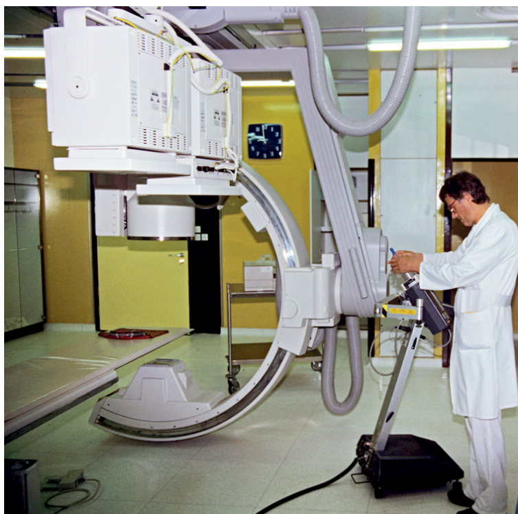
FIGURE 15. Philips-Integris C for digital subtraction angiography (1993–2009) (Marijan Klemenc, Radiol. Ing.)
