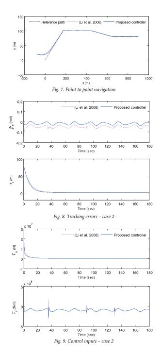
and (650,80). Consequently, the reference trajectory is nonsmooth. Figs. 7–11 present the simulation results. Fig. 7 shows that both control schemes force the underactuated vessel to track the predefined path closely. The position tracking errors converge to small nonzero values at similar rates, as shown in Fig. 8. The proposed controller can effectively reduce the heading error and let it converge to a smaller set.
