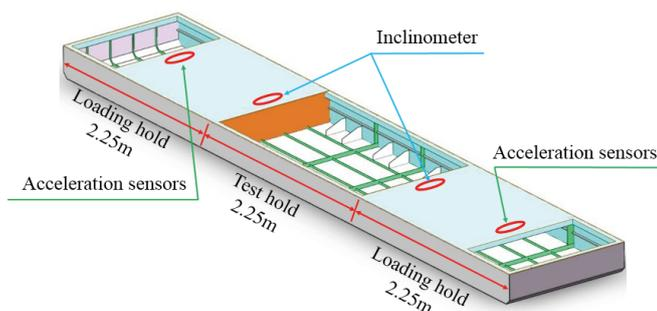
Fig. 3. Measurement point of ship motion
