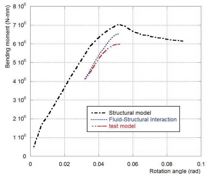
Fig. 13. Comparison on relationship of bending moment and rotation angle
