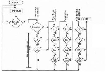
Fig.1. Schematic presentation of the process of checking vulnerability to four stability failure modes (from [6])
