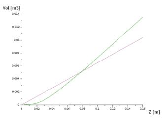
Fig. 4. The graph of the function Vol(z), which defines the water volume displaced by the lifeboat model depending on the draft (green) against the diagram of water displaced by a cylinder with a cross-section such as the average waterline of the model (violet).
