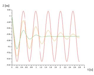
*Fig. 3. The graphs of damped motion depending on the damping factor b value (red: b=0, orange: b=10, green: b=30 ).*
