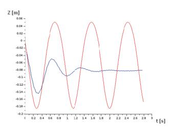
Fig. 5. The numerical solution of equation (3) for m = 5.2kg,  $g=9.81 \text{ m/s}^2$ ,  $\rho_w = 1000 \text{ kg/m3}$  and b = 0kg/s (red) against the results from the experiment (blue).
