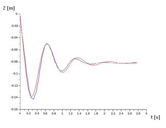
Fig. 6. The numerical solution of equation (4) for m = 5.2kg,  $m_a = 7.5kg$ ,  $g = 9.81m/s^2$ ,  $\rho_w = 1000 kg/m^3$  and b = 44.0kg/s (red) against the results from the experiment (blue).
