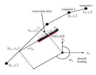
Fig. 4. Schematic diagram for LOS (line of sight)
