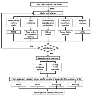
Fig. 1. Diagram of trajectory tracking control system design
