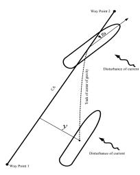
Fig. 3. Diagram of trajectory tracking control
