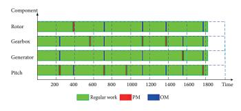
Fig. 6. Grouping maintenance planning with imperfect maintenance for onshore WT system
