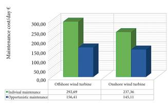
Fig. 7. Maintenance cost comparison between offshore and onshore WTs system
