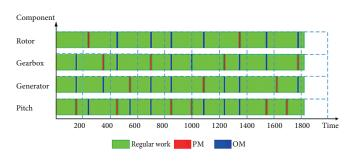
Fig. 4. Grouping maintenance planning for OWTs considering imperfect maintenance
