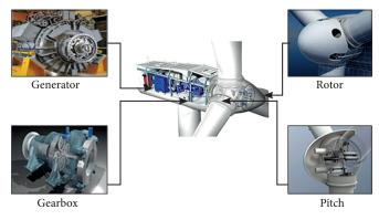
Fig. 1. The critical components of OWT system
