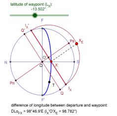
Fig. 16. Result of the graphical method to find the waypoint under condition 3 in example
