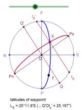
Fig. 15. Result of the graphical method to find the waypoint under condition 2 in example
