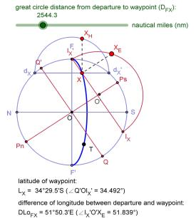
Fig. 14. Result of the graphical method to find the waypoint under condition 1 in example
