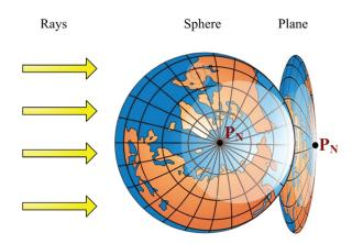
Fig. 3. An illustration of the azimuthal orthographic projection (equatorial aspect)
