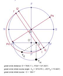
Fig. 13. Result of the graphical method to find the great circle distance and initial course in example
