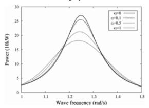
Fig.9. Captured wave power with wave frequencies when  $C_{PTO}=10 \text{ kN/s/m}$
