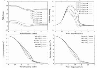
Fig.4. Non-dimensional added mass (upper-left), radiation damping (upperright) and wave excitation force (below) in array layout (a) with incident wave direction ( $\beta = 0^{\circ}$ , 45°) and separating distance (L/R = 0.5, 1.5)
