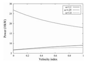
Fig.10. Captured wave power with velocity indexes when  $C_{PTO} = 10 \text{ kN·s/m}$
