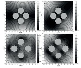
Fig.5. Non-dimensional elevations at the free surface in array layout (a) with incident wave direction ( $\beta = 0^{\circ}, 45^{\circ}$ ) and separating distance (L/R=0.5, 1.5)
