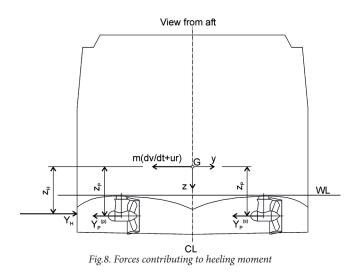
Heeling moment acting on manoeuvring vessel comes from side forces included in the equation of motion (3):
