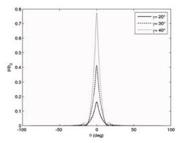
Fig. 4b. Beam patterns in the focal plane Comparison of pressure amplitude for difference frequency wave using SBE model with three different of halfaperture angle
