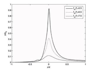
Fig. 3a. On-axis Comparison of pressure amplitude for difference frequency wave using SBE model with three different of downshift ratios
