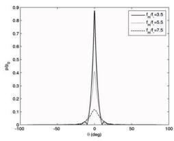
Fig. 3b. Beam patterns in the focal plane Comparison of pressure amplitude for difference frequency wave using SBE model with three different of downshift ratios
