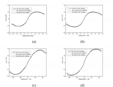
Fig. 9. Measured skeleton curve of specimens: (a) RC-1 specimen (b) RC-2 specimen (c) ST-1 specimen (d) ST-2 specimen
