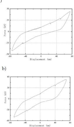
Fig. 6. Hysteretic circle of the ST specimen in destruction: (a) ST-1 specimen (b) ST-2 specimen
