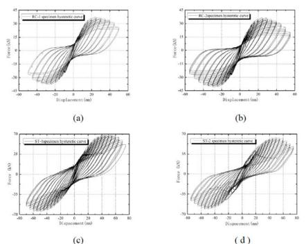
Fig. 8. Measured force - displacement cyclic response of specimens: (a) RC-1 specimen (b) RC-2 specimen (c) ST-1 specimen (d) ST-2 specimen
