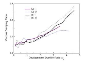
Fig. 11. The equivalent viscous damping ratio of specimen
