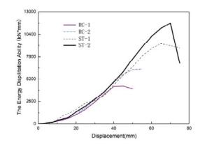
Fig. 10. The dissipated hysteretic energy capability of specimen
