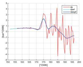
Fig. 12. Derivatives of curves smoothed using the low-pass filter with cut-off frequency of 800 Hz (dpf) and the Savitzky-Golay filter (dpwg4)
