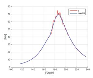
Fig. 3. Indicator curve smoothed using the moving average method with the moving interval consisting of k = 20 points (pwm20), as compared to the original curve (p)
