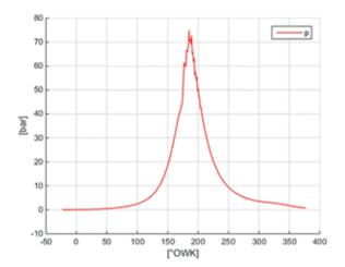
Fig. 2. Indicator diagram of the engine Al 25/30
