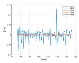
Fig. 14. Disturbances extracted in four successive steps of p curve approximation making use of the 3rd order polynomial with z K=16 (Fig.1).
