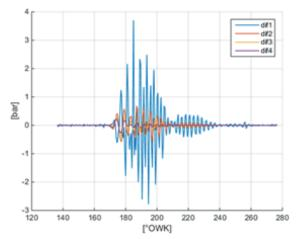
Fig. 13. Disturbances extracted in four successive steps of p curve approximation making use of the 3rd order polynomial with K=12 (Fig. 1).
