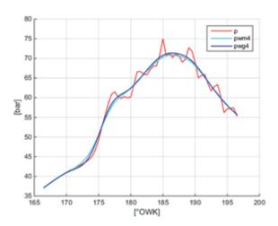
Fig. 7. Indicator curve smoothed using the moving average method with the interval consisting of k=5 points (pwm4), and the Savitzky-Golay filter with the interval consisting of k=12 points (pwg4). In both cases smoothing was repeated four times.
