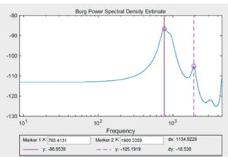
Fig. 15. Amplitude spectrum of disturbances extracted after step 1 of smoothing. Angle interval from 80 to 140° OWK.
