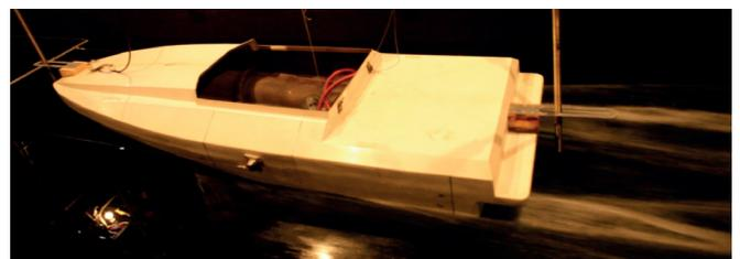
Fig. 8. High-speed navigation at 13 m/s without air jets
