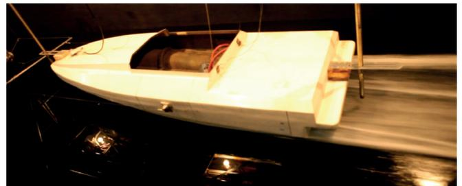
Fig. 7. High-speed navigation at 13 m/s with air jets
