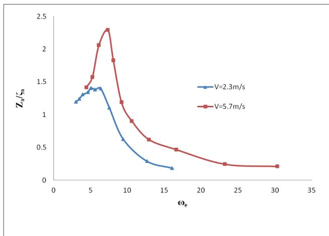
Fig. 11. Heave curve of the trimaran planing boat in waves
