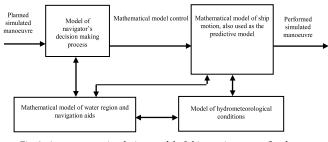
Fig. 3. Autonomous simulation model of ship motion on confined water regions
