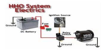
Fig.3. Schematic diagram showing how HHO system is included into electric network of a car
