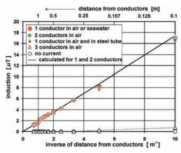
Fig. 3. Electromagnetic field (expressed by magnetic component – induction) around AC conductors
