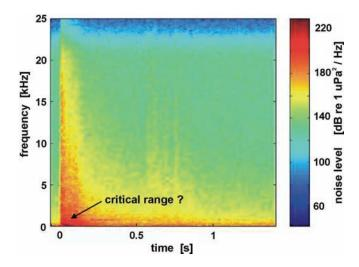
Fig. 6. Sample modification of the acoustic field by the noise generated by activities during wind farm construction (at a distance of 1881 m). Vertical axis represents the acoustic frequency, while the horizontal axis shows the time elapse.
