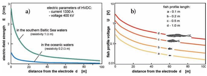
Fig. 4. Electric field generated by the electric current flowing in the seawater depth (a) and fish profile voltage in this field (b) in the vicinity of the electric power transmission system electrode in HVDC solution (relations calculated by authors using the model in which the electrode surface S = 450 m2 is represented by the surface of an equivalent sphere).
