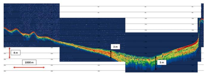
Fig. 14. Echogram taken along the transect marked on the geological map (Fig. 13)
