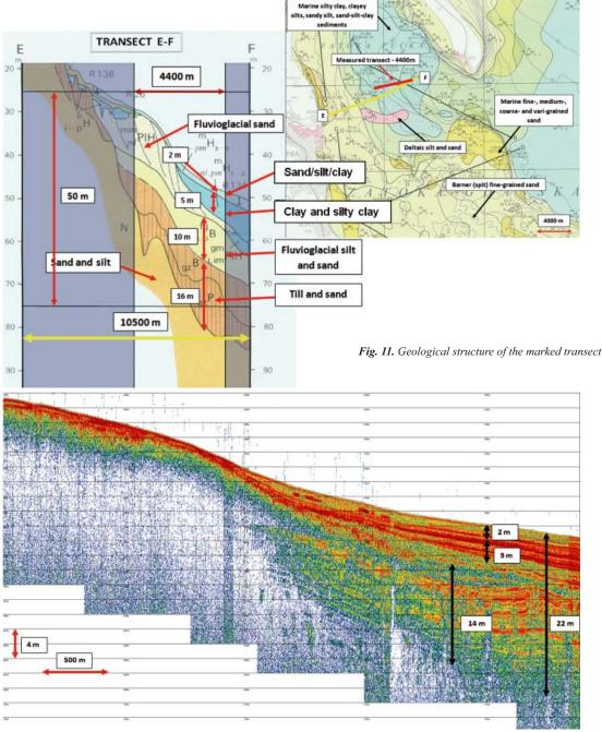
Fig. 12. Echogram taken along the transect marked with red line in Fig. 11
