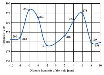
Fig. 8. Hardness distribution across W2.1 test joint of S500M steel welded underwater, HVmax = 283
