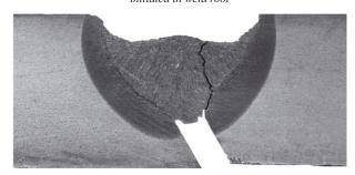
Fig. 4. Cross section of the 1A (S355J2G3) test joint with the visible crack initiated in fusion line
