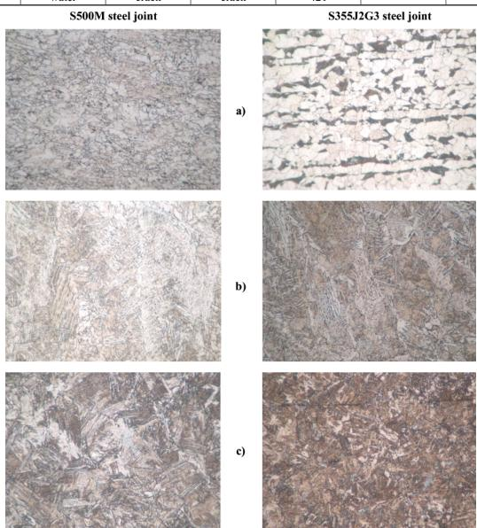
$\textbf{\textit{Fig. 6.}} \textit{ Microstructure of S500M and S355J2G3 steel joints welded underwater; \textbf{\textit{a})} \textit{ base material, \textbf{\textit{b})} weld, \textbf{\textit{c})} \textit{ overheated zone in HAZ. Magnification} \times 200$
