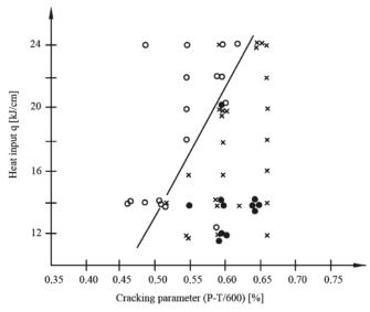
Fig. 2. Results of Tekken tests, underwater wet MMA welding: ○ – no cracks, × – internal cracks, • – internal and external cracks [4]
