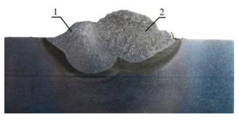
Fig. 10. Cross section of the test weld beads; S355J2G3steel; 40% pitch
