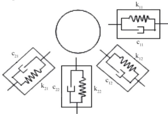
Fig. 8. Stiffness and damping coefficients the oil film
