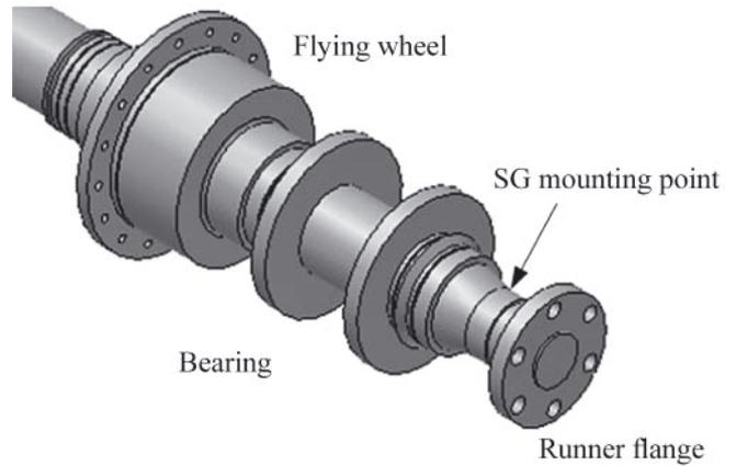
Fig. 5. Strain gages position in the shaft
