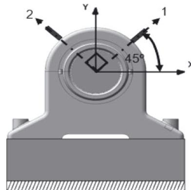
Fig. 9. Place of the sensors on the rotor
