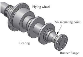
Fig. 5. Strain gages position in the shaft
