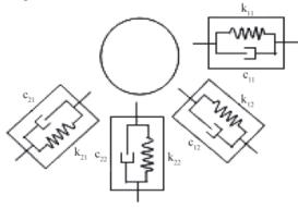
Fig. 8. Stiffness and damping coefficients the oil film
