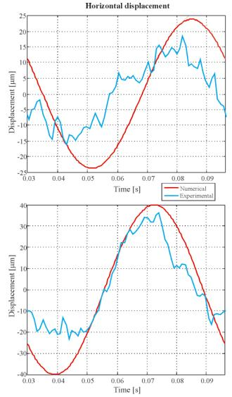
Fig. 12. Numerical and experimental displacement signals for the bearing 2
