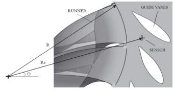
Fig. 2. Position of the sensors
