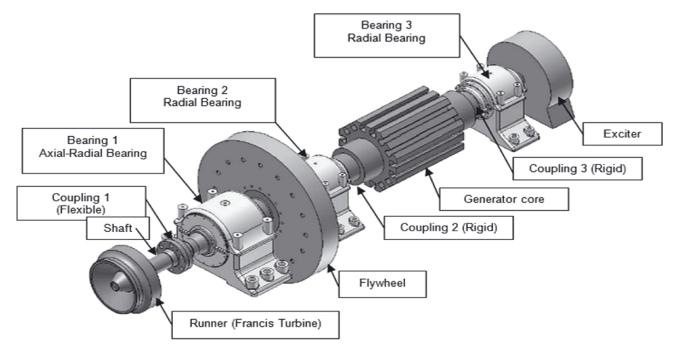
Fig. 1. Turbine shaft with bearings and attached mechanical elements
