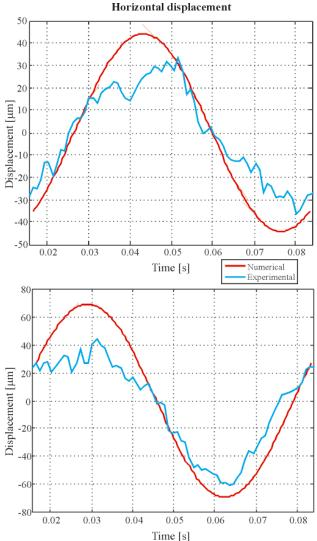
Fig. 11. Numerical and experimental displacement signals for the bearing 1
