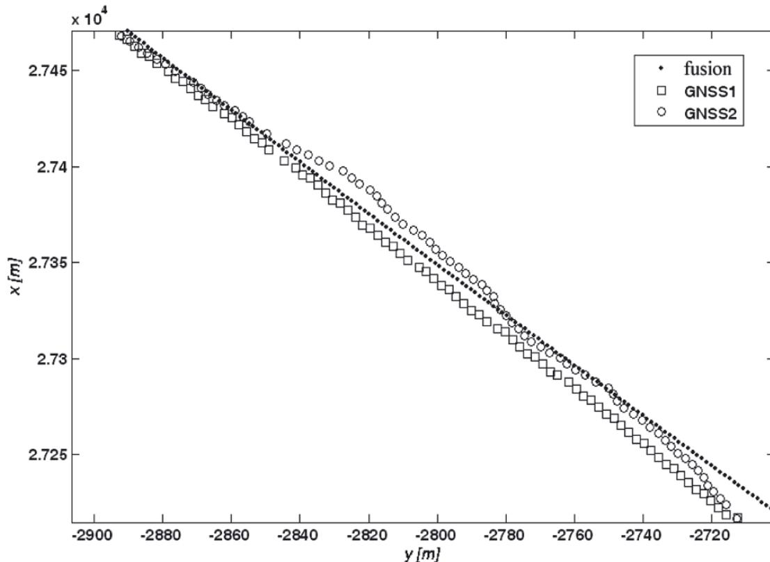
Fig. 5. Ship's positions measured by GNSS<sub>1</sub> and GNSS<sub>2</sub> receivers and the measurement fusion – situation 2
