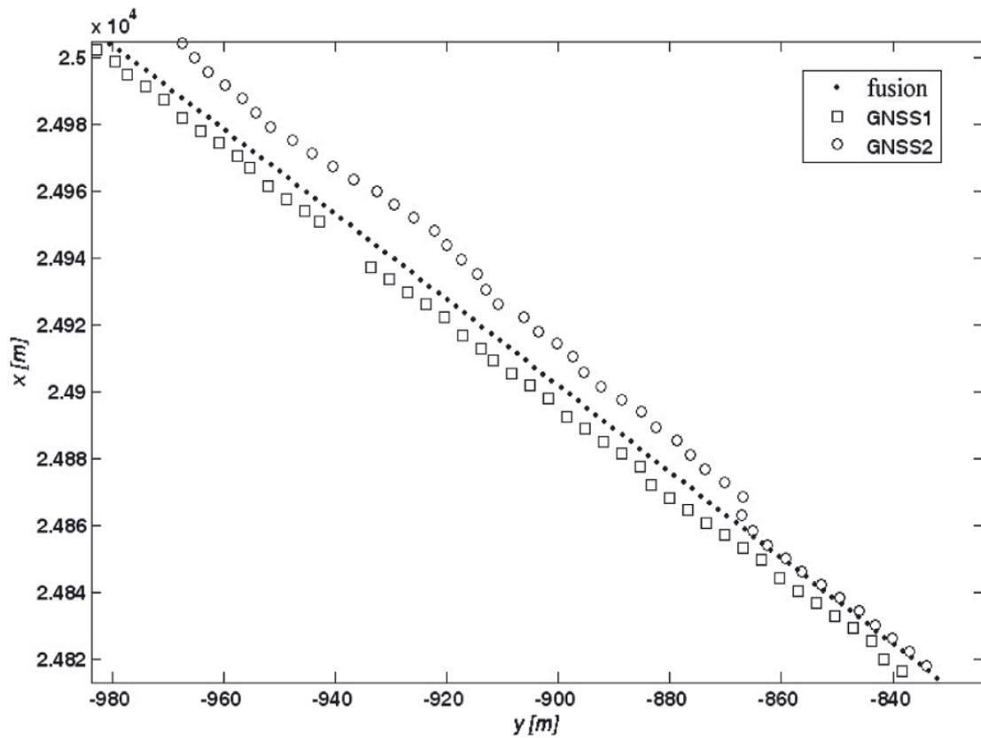
Fig. 6. Ship's positions measured by GNSS<sub>1</sub> and GNSS<sub>2</sub> receivers and the measurement fusion – situation 3
