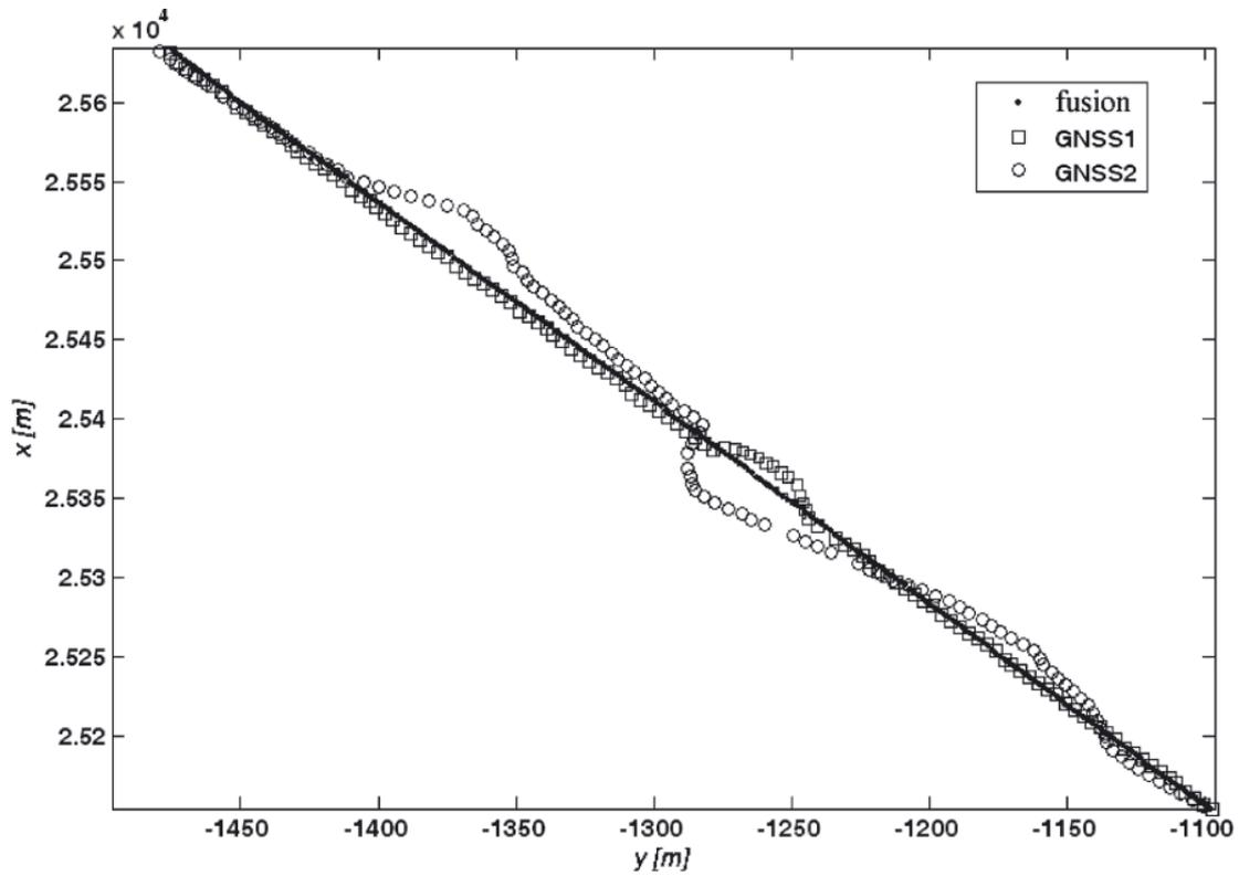
Fig. 4. Ship's positions measured by GNSS<sub>1</sub> and GNSS<sub>2</sub> receivers and the measurement fusion – situation 1
