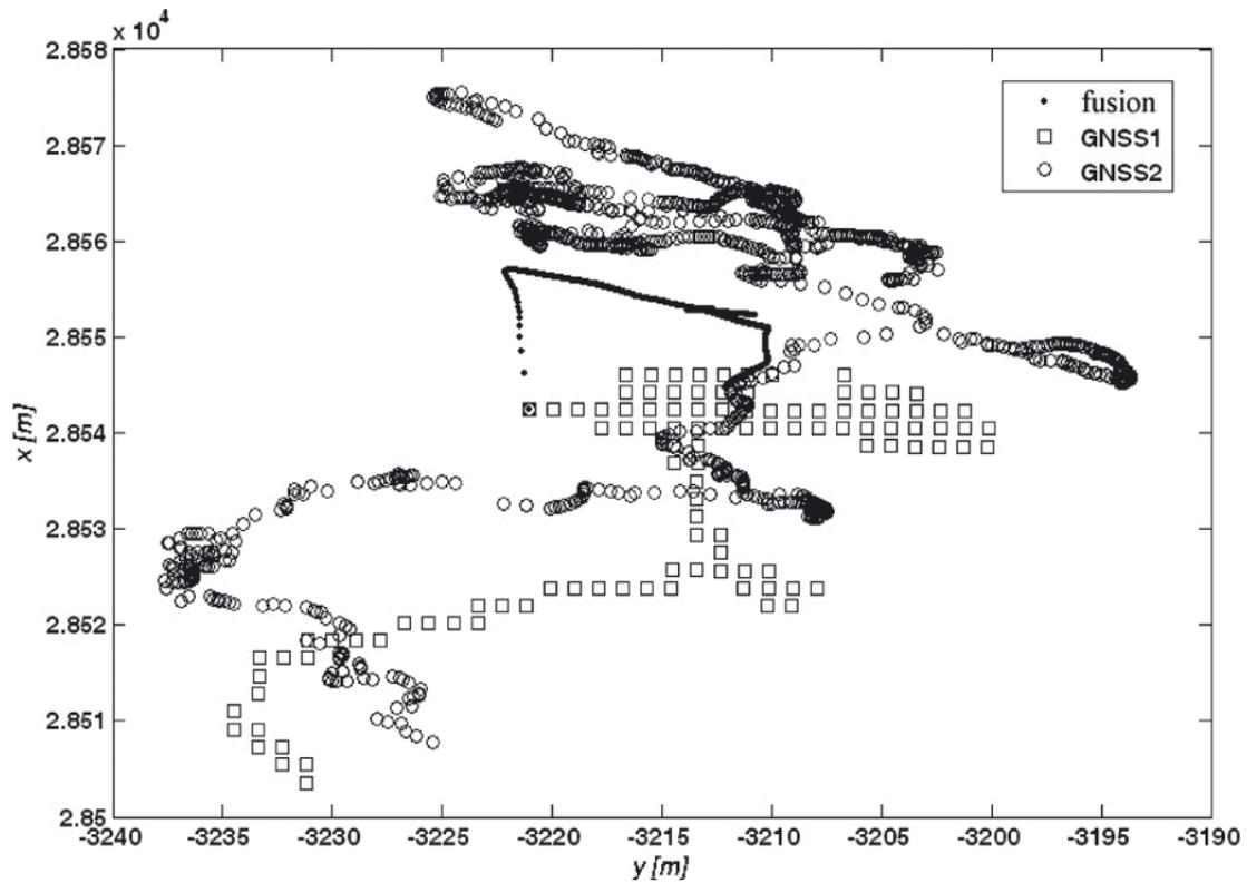
Fig. 7. Ship's positions measured by GNSS<sub>1</sub> and GNSS<sub>2</sub> receivers and the measurement fusion – situation 4
