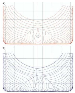
Fig. 1. Body lines of stern part of B 573 ship hull: a) before modification (symmetric stern), b) after modification (asymmetric stern)
