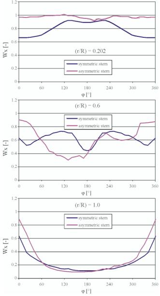
Fig. 5. Distribution of the axial wake fraction  $W_x$  for both the symmetric and asymmetric stern, given at the values of the relative radius (r/R) = 0.202; 0.6; 1.0
