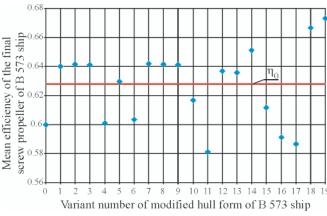
Fig. 6. Mean efficiency of the final screw propeller of B 573 ship, operating in non-homogenous wake current field. Notation: η<sub>0</sub> – maximum efficiency of the final screw propeller in homogenous water velocity field (free propeller); Variant No.0 – the initial hull form of B 573 ship (without modification), wake current field - as measured during model tests;
