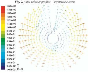
Fig. 3. Velocity vectors – asymmetric stern
