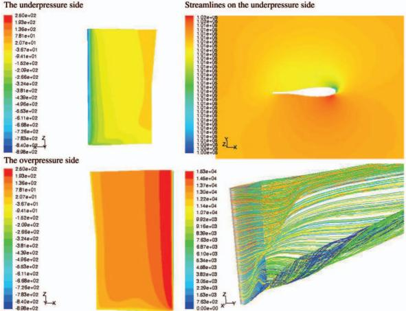
Fig. 9. The pressure distribution and streamlines for 40° angle of attack (the rudder of IFS58-TR15 profile)
