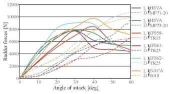
Fig. 11. Values of the lifting force L and drag force D versus rudder angle for the considered rudders
