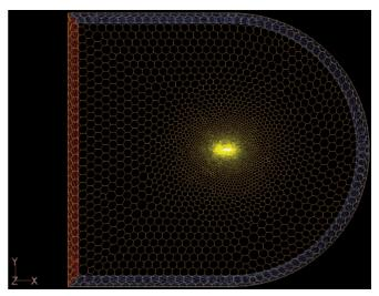
Fig. 6. The computational domain mesh. Notation: the blue area – velocity inlet, the yellow one – plane of symmetry, the red one – pressure outlet
