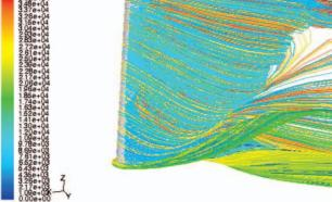
Fig. 12. The pressure distribution and streamlines for the IFS58-TR15 profile rudder at 40° angle of attack
