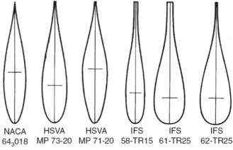
Fig. 1. The profiles used for the investigated rudders
