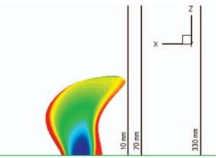
Fig. 4. Location of the cross-sections of the tip vortex for computations and measurements
