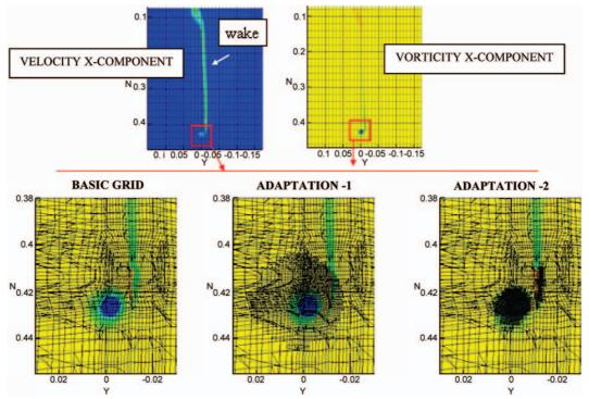
Fig. 8. Process of grid refinement in the tip vortex area
