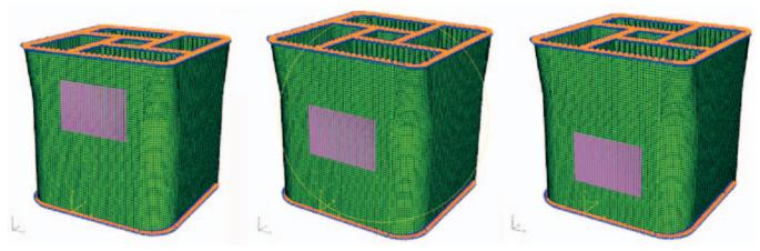
Fig. 3. Column c1 south wall. Wave slamming pressure exposed area A1 -A3
