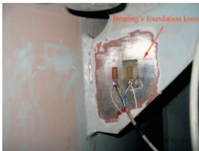
Fig. 4. Stress measurement of bearing's foundation knee
