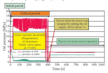
**Fig. 16.** Oil pressures at motor inlet and outlet: cold chamber temperature  $t_{ol} = -15$  [°C], oil temperature  $t_{ol} = 53$  [°C], the oil flow rate Q = 100 [l/min]
