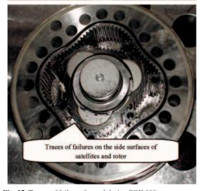
Fig. 17. Traces of failures formed during SOK 100 motor start-up with symptoms of incorrect operation in thermal shock conditions
