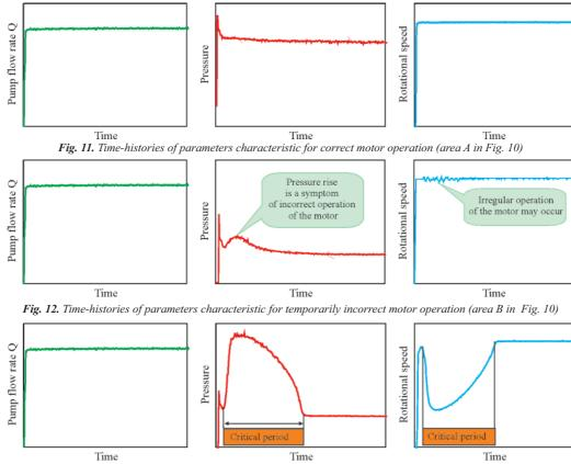
Fig. 13. Time-histories of parameters characteristic for incorrect motor operation (area C in Fig. 10)
