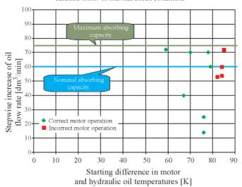
Fig. 19. Starting parameters of GMR 160 motor in thermal shock conditions
