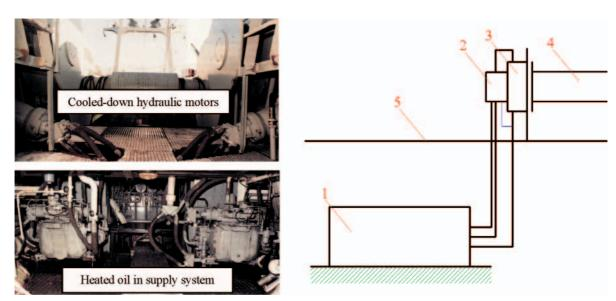
Fig. 2. Simplified schematic diagram of supplying the hoisting winch: 1 – ship's central oil supply system, 2 – set of valves, 3 – hydraulic motor, 4 – hoisting winch, 5 – ship's deck
