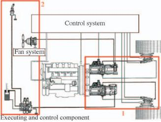
Fig. 3. Hydraulically driven bulldozer: 1 – travelling system, 2 – working unit and fan systems [10, 11]
