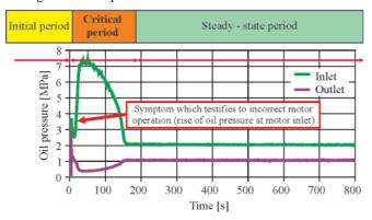
**Fig. 15.** Oil pressures at motor inlet and outlet: cold chamber temperature  $t_{oi} = -20$  [°C], oil temperature  $t_{oi} = 50$  [°C], oil flow rate Q = 100 [l/min]
