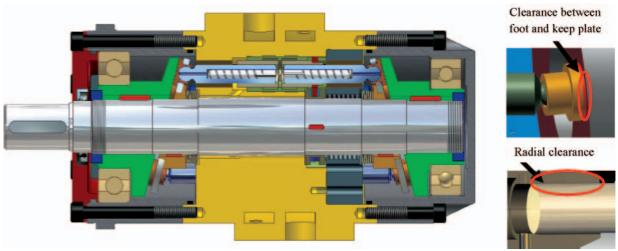
Fig. 4. PWK 27 axial piston pump [5] with indicated places between co-operating elements where the disappearance of the clearance can occur
