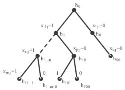
**Fig. 3.** Way of elaborating the solution tree for the knapsack problem by means of searching method with reversals. Numbers given at nodes correspond to values of the coefficient which determines the assignment of i-th task to j-th operator in the considered schedule harmonogramie  $h_{n,n}$ :
