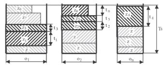
Fig. 2. The example showing the assignment of operational tasks to three operators, i.e. packing three different knapsacks
