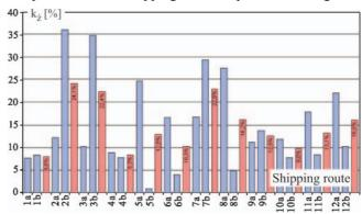
Fig. 27. The service margin  $k_z$  calculated for K1 ship in function of shipping route, for  $V_{ZE} = V_K$  and  $P_{VE} = 0.95$ ; blue - service margin for one-leg voyage of the ship; red - mean service margin for a shipping route .
