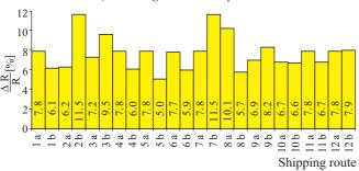
Fig. 19. Index of additional resistance increase for K1 ship, depending on shipping route.
