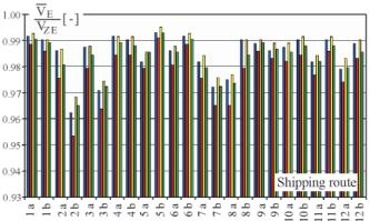
Fig. 21. Index of maintaining the set service speed  $V_{\rm ZE}$  of bulk carriers blue - M1; red - M2; yellow - M3; green - M4.
