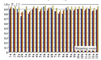
Fig. 23. Probability of maintaining the set service speed  $V_{\rm ZE}$  of containerships : blue - K1; red - K2; yellow - K3.
