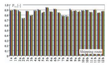
Fig. 20. Probability of maintaining the set service speed  $V_{\rm ZE}$  of bulk carriers : blue - M1; red - M2; yellow - M3; green - M4.
