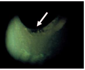
d) Outlet valve seat of Wartsila engine – carbon deposit layer close to valve seat face – exhaust gas blow-by through non-tight valve
