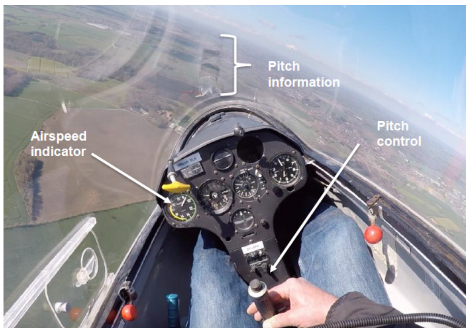
Figure 2. Airspeed information and control in a first-person perspective.
