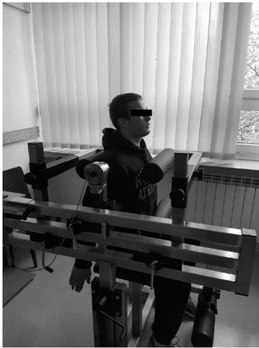
**Figure 3.** Measurement of the torque of the shoulder muscles in static conditions
