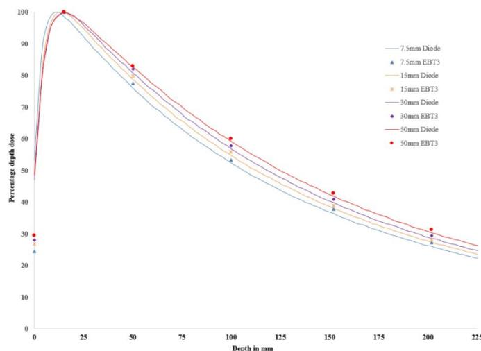
**Figure 7b.** PDD: Diode P versus EBT3 film for 7.5 mm, 15 mm, 30 mm, 50 mm collimators.
