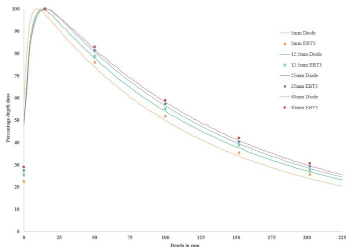
**Figure 7a.** PDD: Diode P versus EBT3 film for 5 mm, 12.5 mm, 25 mm, 40 mm collimators.
