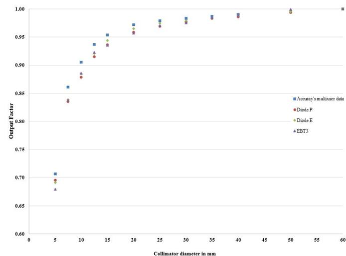
**Figure 1.** Comparison of output factors measured by diode P, diode E, EBT3 film detectors and Accuray multiuser data.
