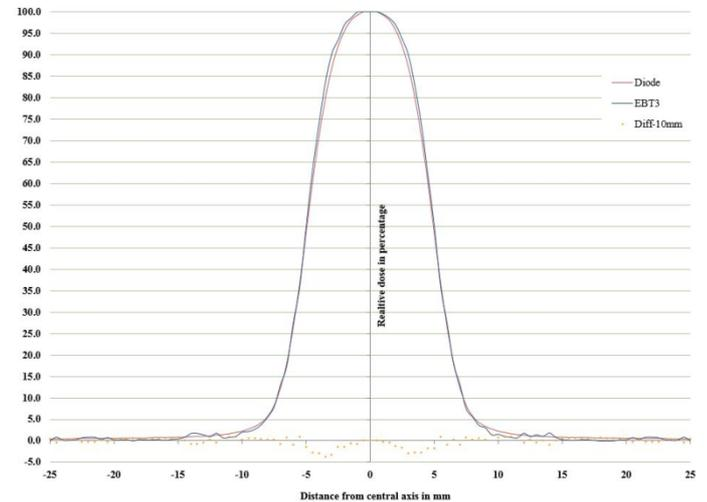
**Figure 4.** Diode P versus EBT3 film OCR profile with relative dose difference in percentage for 10 mm collimator.
