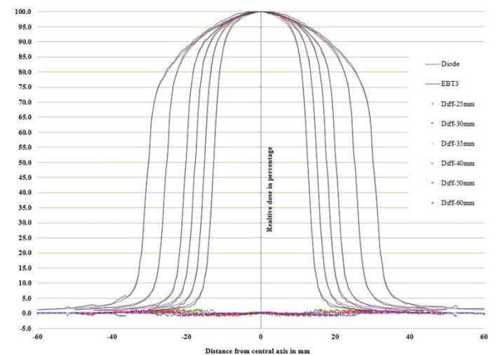
**Figure 6.** Diode P versus EBT3 film OCR profile with relative dose difference in percentage for 25 mm, 30 mm, 35 mm, 40 mm, 50 mm, 60 mm collimators.
