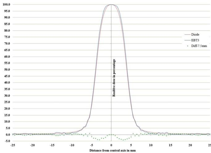
**Figure 3.** Diode P versus EBT3 film OCR profile with relative dose difference in percentage for 7.5 mm collimator.
