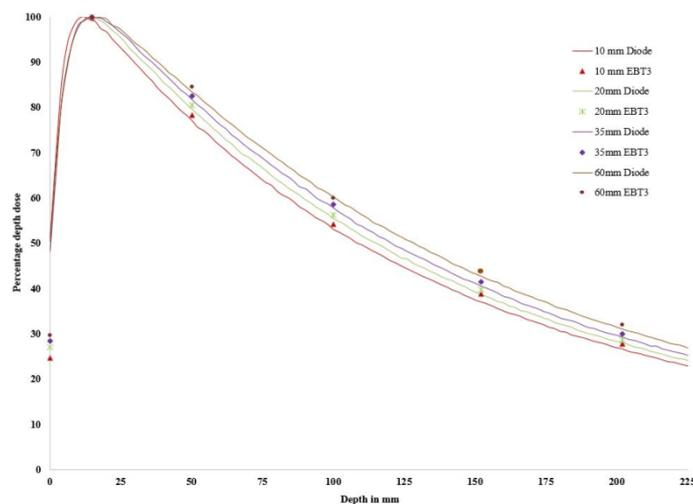
**Figure 7c.** PDD: Diode P versus EBT3 film for 10 mm, 20 mm, 35 mm, 60 mm collimators.
