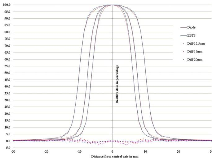
**Figure 5.** Diode P versus EBT3 film OCR profile with relative dose difference in percentage for 12.5 mm, 15 mm, 20 mm collimators.
