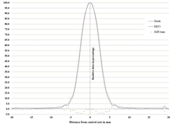
**Figure 2.** Diode P versus EBT3 film OCR profile with relative dose difference in percentage for 5 mm collimator.
