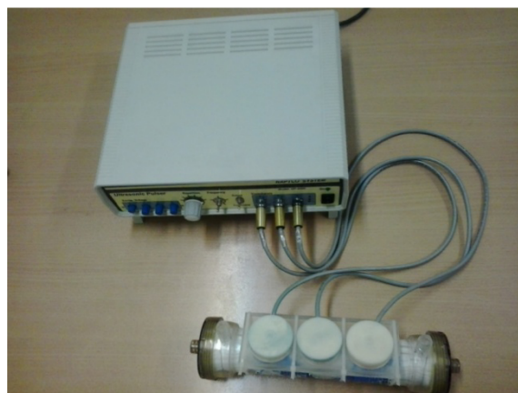
Figure 1. Photo of three transducers mounted on a Plexiglas plate and placed at a distance of 5 mm from the dialyzer housing.
